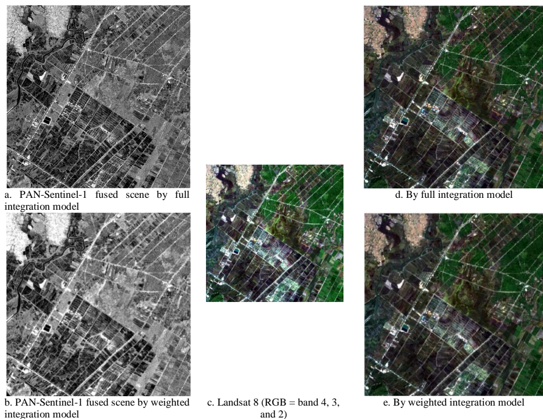
Fig. 5. Fusion results of Sentinel-1 and Landsat 8 using FI model, WC model with PCA-wavelet fusion method
